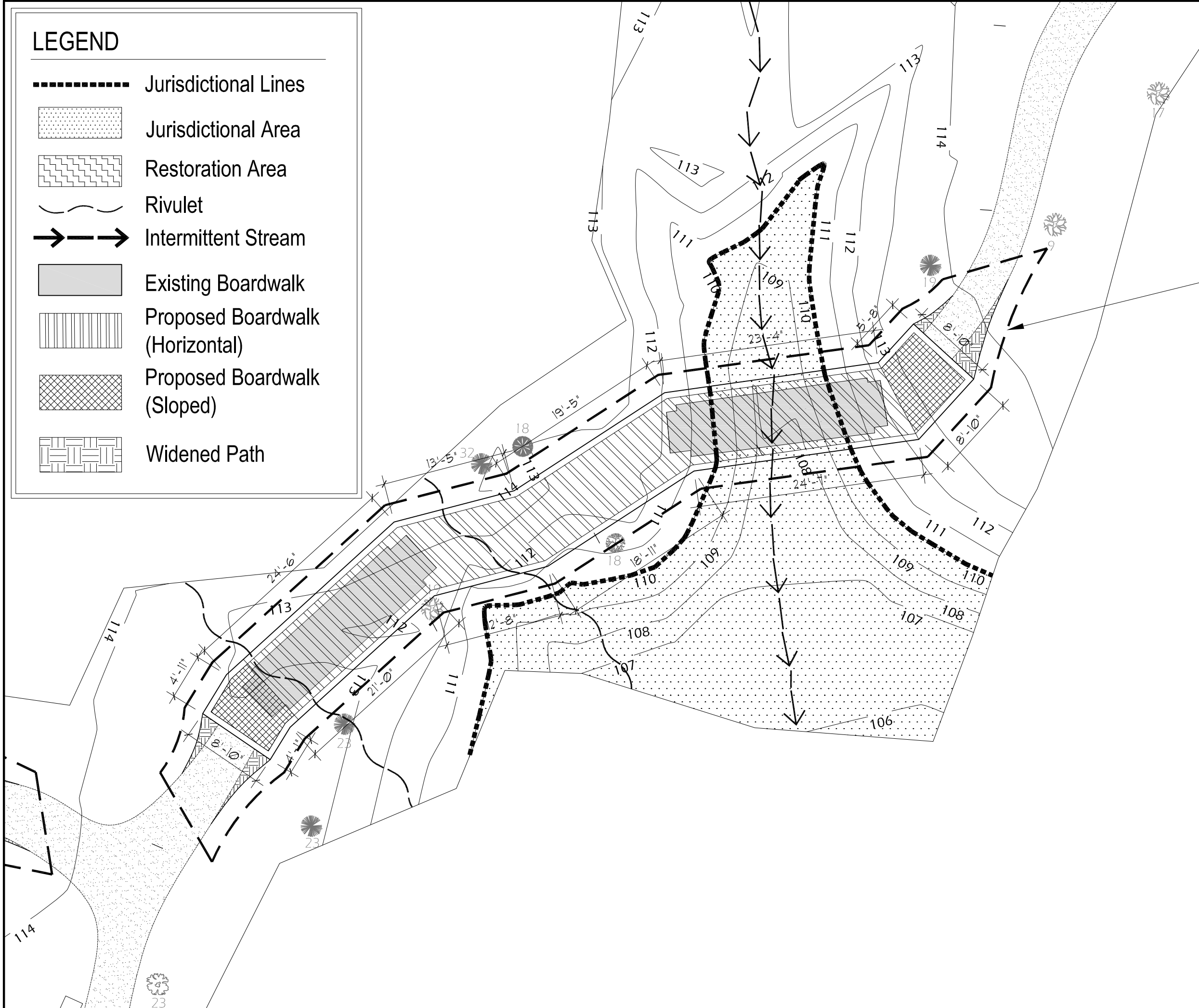
4 NEW BOARDWALKS 3 AND 5 SCALE: 1" = 10'-0"
