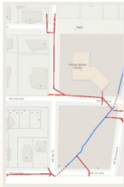
Figure 9: Existing Off-Site Storm System
