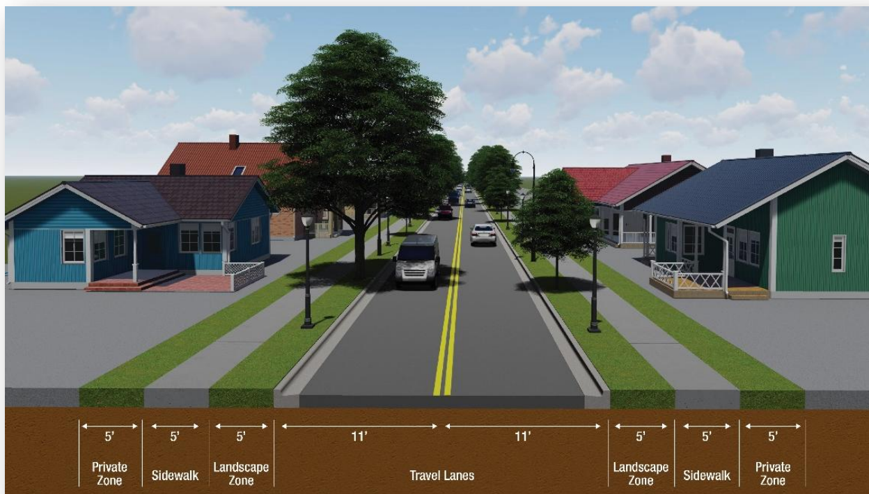
Figure 9: Suburban-Type Development Typical Section
