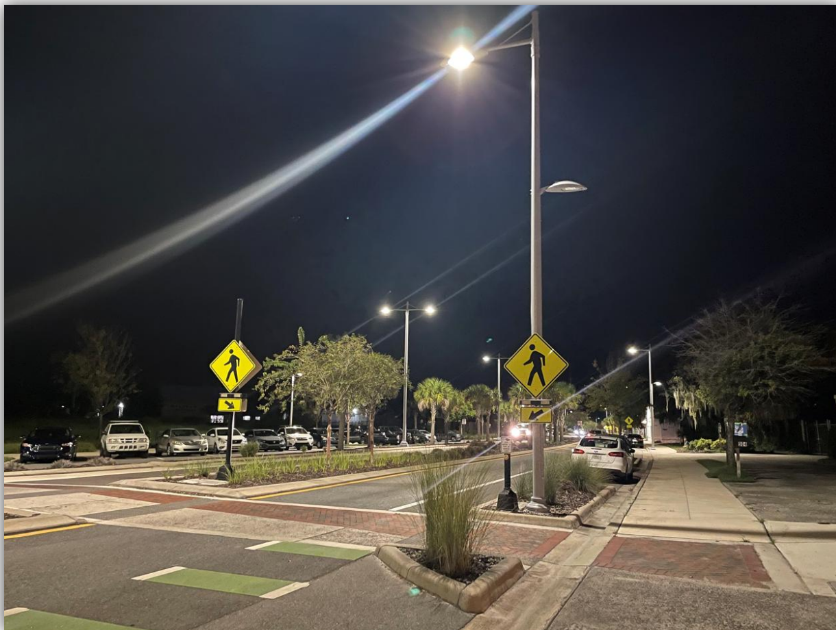
Figure 6: Main Street Pedestrian and Roadway Lighting on a Single Pole (Near 900 S Main Street)
