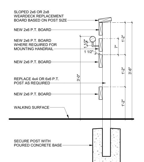
8 TYPICAL REPLACEMENT RAILING SECTION
